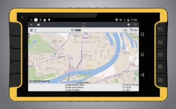
LT600 series can work either as a GNSS controller with big display, or a tablet with enhanced accuracy for GIS data collection. It is compatible with CHC LandStar 7 software and GIS Apps on Google Play.
